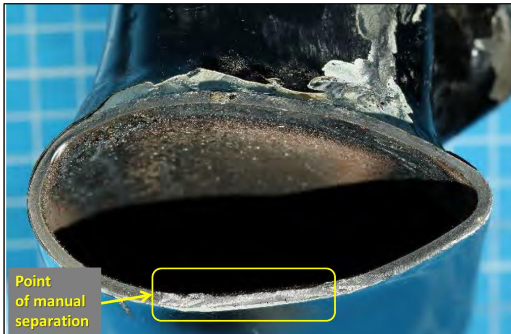
Photo No. 9: Fracture point of the diagonal brace with the housing
