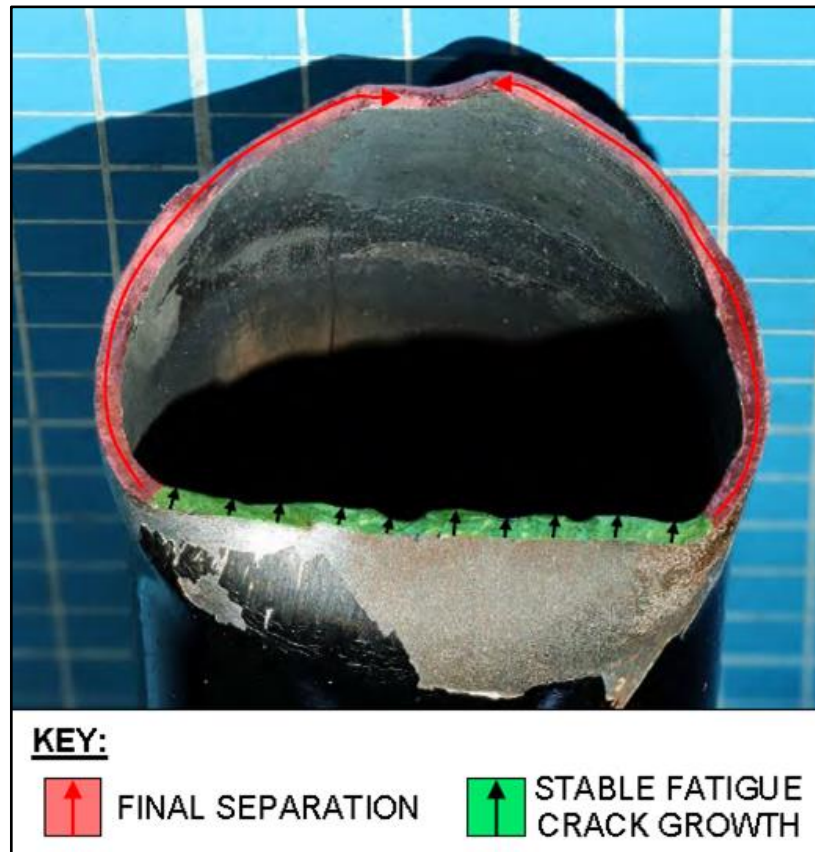
Photo No. 10: Failure sequence of the inboard horizontal tube
